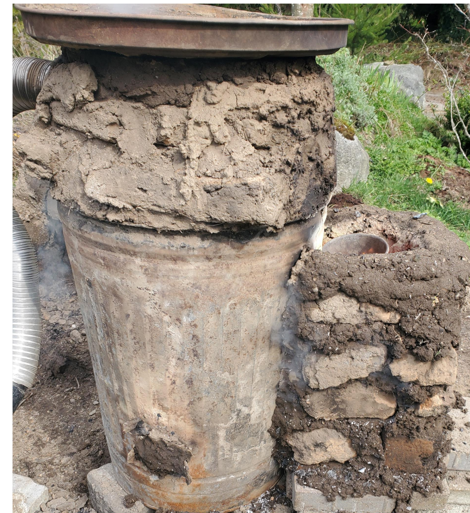
Figure 2. Side view of blast furnace with wood chamber on left and crucible chamber on right. An air intake tube is attached to the top of the wood chamber.
