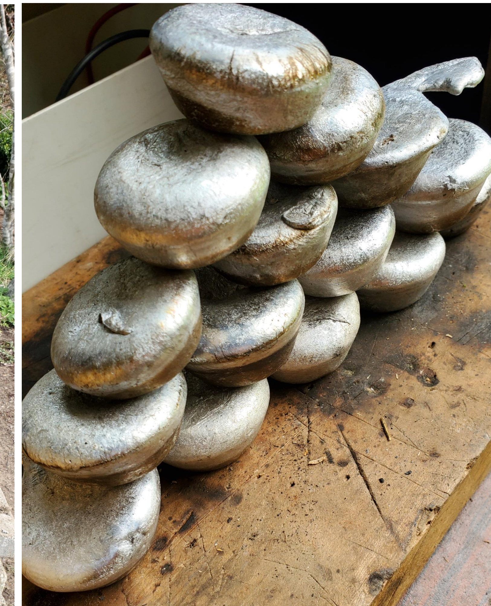
Figure 3. Aluminum ingots created by melting aluminum and pouring it into muffin mold.
