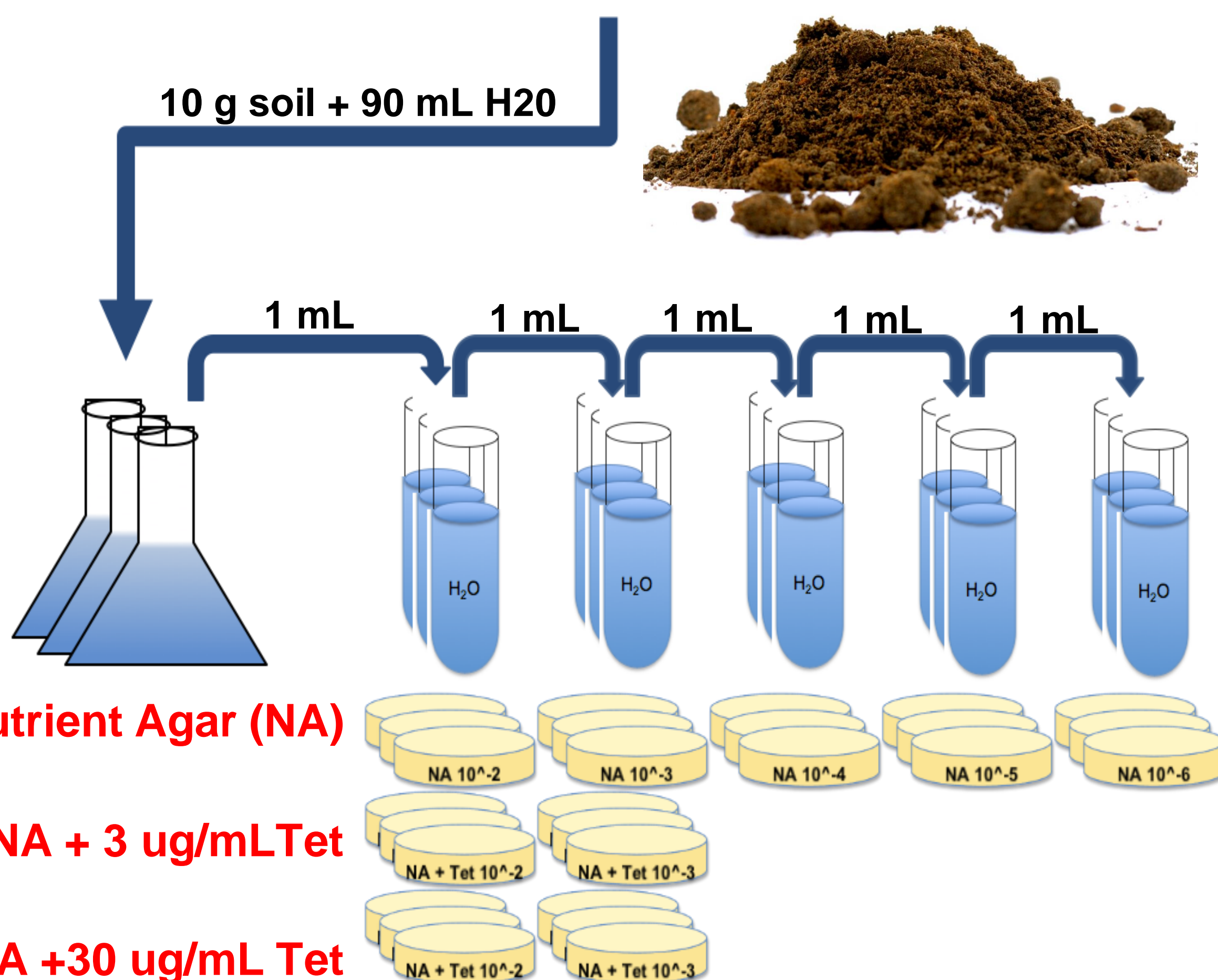
Fig. 1. Nutrient Agar (NA), NA + 3 ug/mL tetracycline, and NA + 30 ug/mL tetracycline plates inoculated with soil dilutions.
