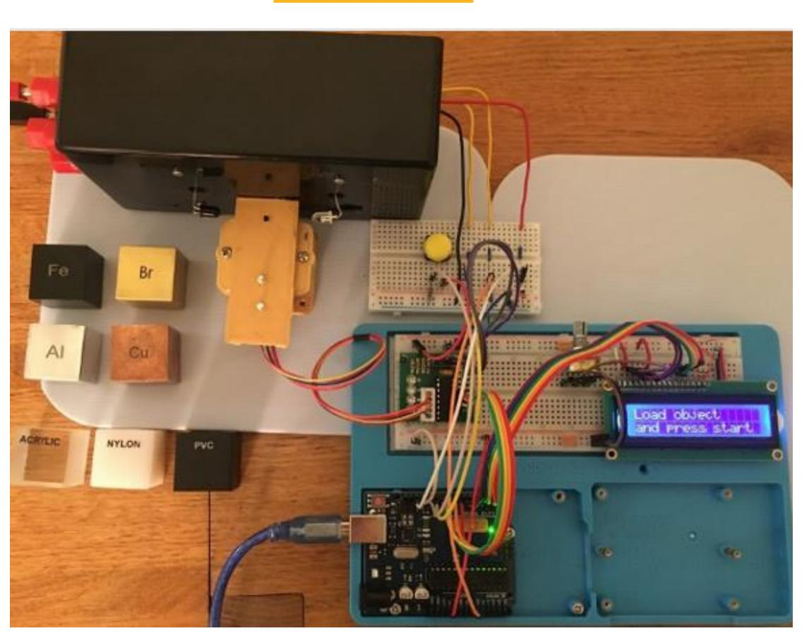
The above circuit accomplishes the objectives of this project. It is able to differentiate between each of the different materials and can also detect when no object is present.
