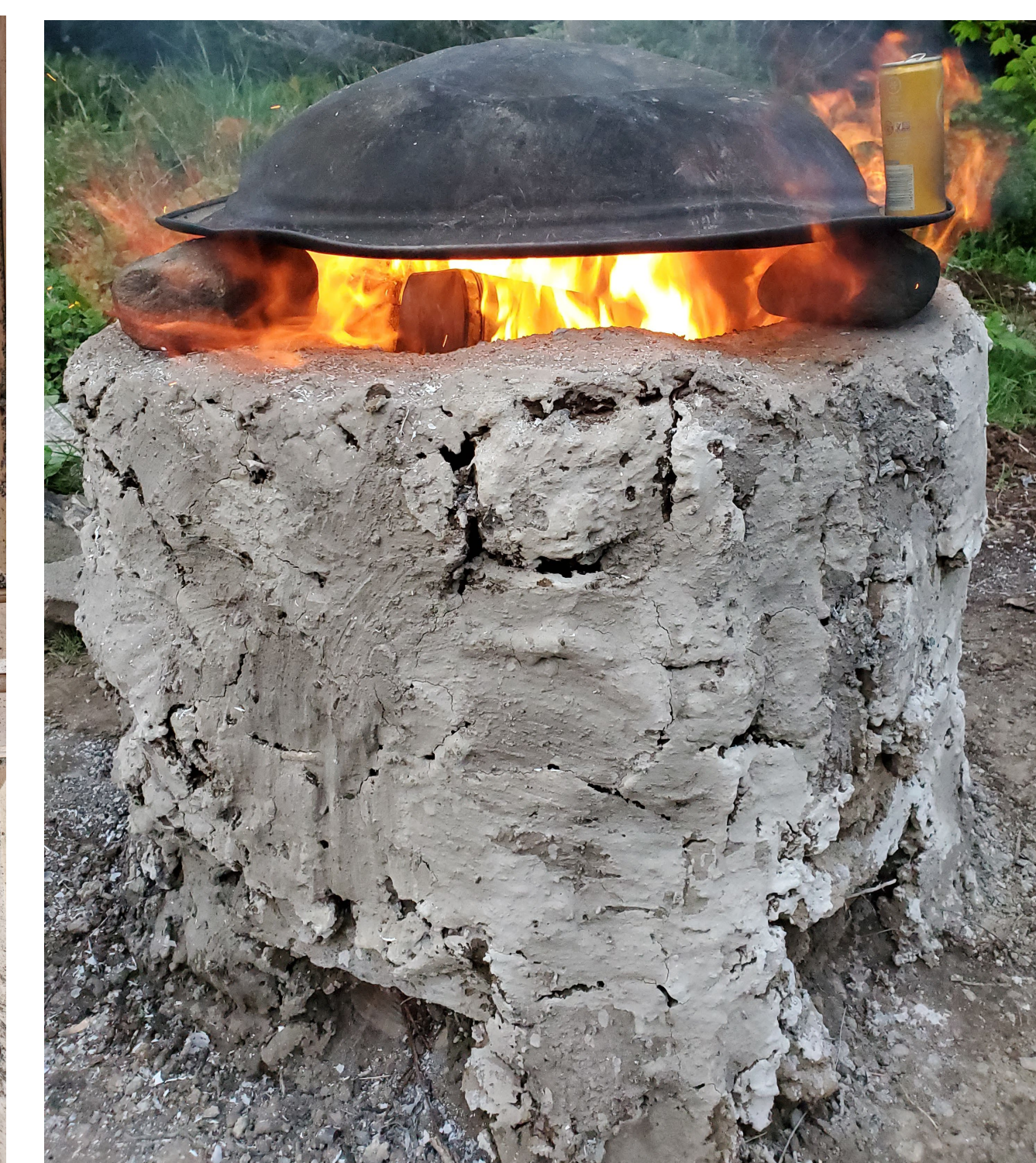
Figure 2. A clay brick furnace processing wood into charcoal. Wood ash paint was applied to provide water resistance. The soda can is for scale.
