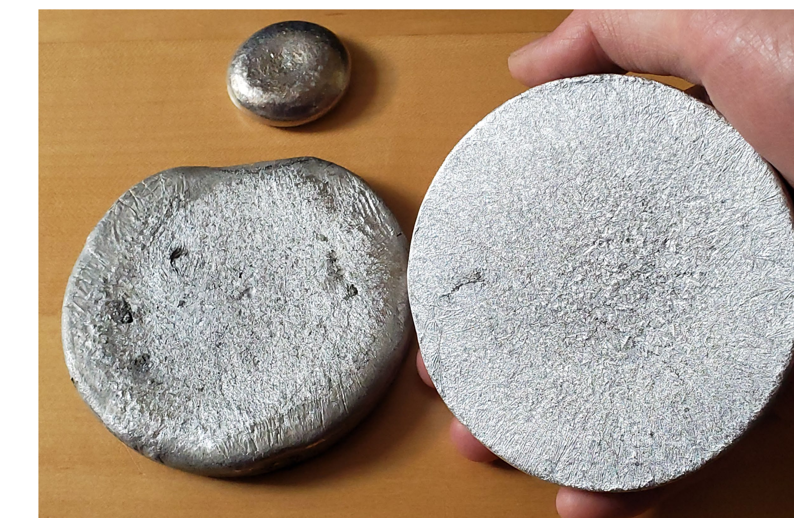
Figure 5. Two aluminum ingots below an aluminum droplet. The ingot on the right is held in hand for scale.
