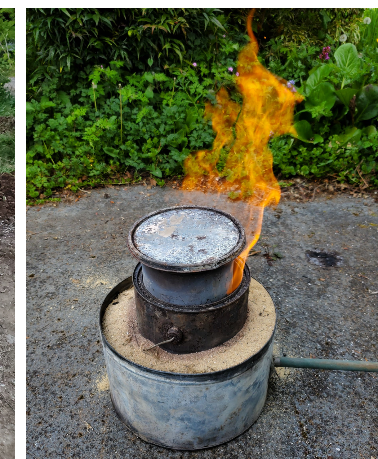
Figure 3. An aluminum melting furnace running at roughly half capacity. The inner diameter is roughly 6 inches.
