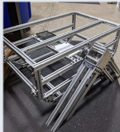
Staging the chassis components: rover body, one arm pair assembly, and temporary mountings for the control system.
