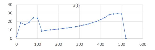
Between **t=0-120** sec, the Shuttle loses mass due to burning the propellent in the booster.
