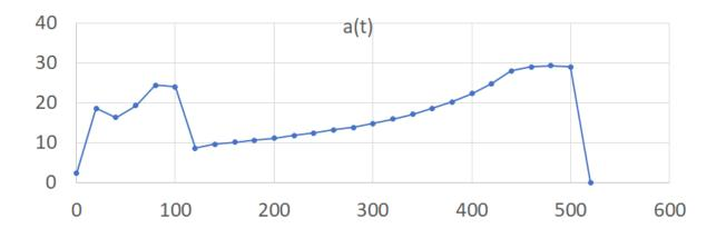
At 120 seconds the space shuttle has burned all the propellant from the SRB and they separate from the space shuttle. By burning more propellant in the external tank (reducing mass), the acceleration increases; and as the mass continues to decrease the acceleration increases at a faster rate until the space shuttle reaches its maximum acceleration of **3 g (29.4 m/s2)** at 450 seconds.
